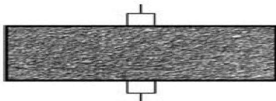
Figure 1. Direct transmission
